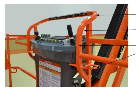
Older-styled platform ---notice shape of railing at control box, plus lanyard attach points
