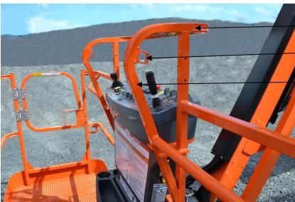
**Newer-styled platform** --- different curvature in railing plus tabs
